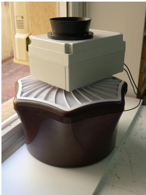
**Figure 62: Mounted trap with the counter and identifier module**
