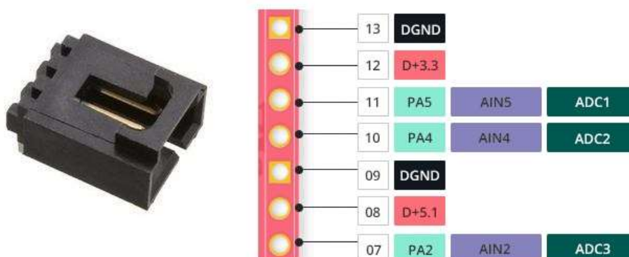
Figure 96: Zolertia Re-mote's analog connector pin-out
