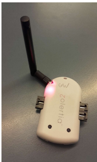
Figure 67: A Zolertia RE-Mote device with its led switched on in red
